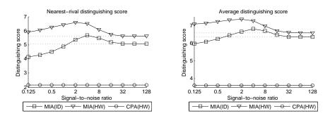
Fig. 3: The effect of Gaussian noise on HW and ID attacks against HW leakage of the first DES S-Box.
