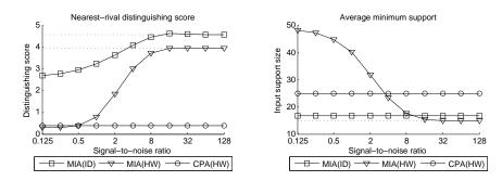
**Fig. 5:** Nearest-rival distinguishability and required support size of theoretic attacks against Hamming distance leakage (with a reference state of  $0100_{(2)}$ ) for varying levels of Gaussian noise.
