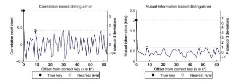
**Fig. 1:** Ideal distinguishing vectors using the HW power model against the output of the first DES S-Box.
