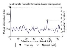
**Fig. 2:** Ideal MIA vector against the DES AddRoundKey and the first S-Box jointly.
