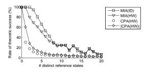
**Fig. 4:** Ideal success against the first DES S-Box in the presence of datadependent reference states of length 8 bits, as the number of different states increases.
