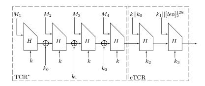
Fig. 2. Example of an eTCR domain extension function for  $H: \{0,1\}^{128} \times \{0,1\}^{640} \rightarrow \{0,1\}^{256}$ .
