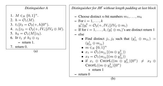
**Fig. 6.** 6(a): Distinguisher for JH-*n* without length padding, 6(b): Distinguisher for JH' without length padding
