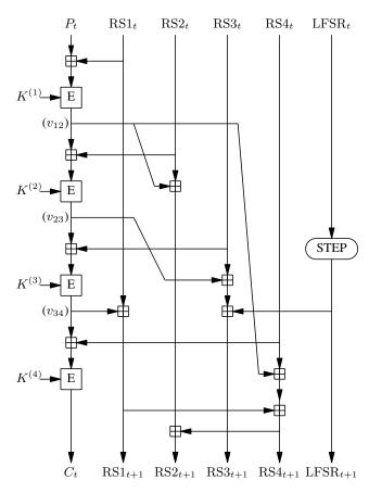
**Fig. 2.** Encrypting a single 16-bit word  $P_t$  to produce a ciphertext word  $C_t$  with Hummingbird. After initialization  $t \ge 0$ .
